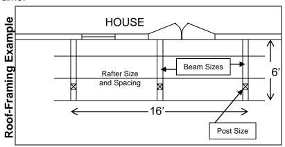
A <u>Cross Sectional Drawing</u> that shows the size and type and spacing of all materials to be used.
